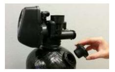
Dome hole tanks are standard for easy replacement of the neutralizing media. Tanks are available in black or natural.
