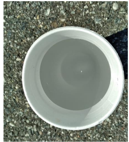
Use a white Styrofoam cup to see if the carbon fines are still in the water. If so, keep flushing!
