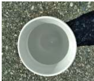
Check closely for carbon fines.
