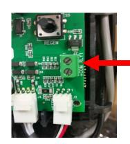
Connect wires from chemical pump here.
