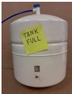
Checking pressure in storage tank. 7 psi is required.
