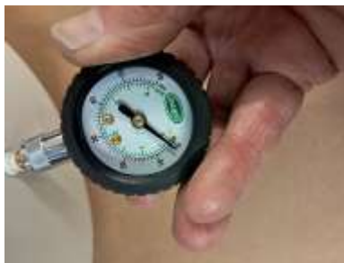
Checking pressure in storage tank. 7 psi is required.
